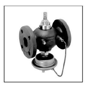
Combined with an electric actuator the AIQM controller is a self-acting flow controller with integrated control valve. The pressure difference across the control valve is kept constantly at 0.2 bar.
